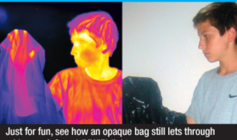
Just for fun, see how an opaque bag still lets through mid-wave infrared (MWIR) light.
